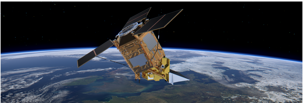
Figure 1.1: Sentinel-5p carrying the TROPOMI instrument measuring air quality. ©ESA/ATG medialab
